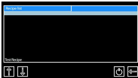
5. The test recipe is found at the bottom of the list; press the downward arrow until you see the recipe.
