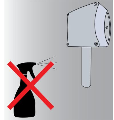
Before beginning, be sure to remove all food product and Maturmeat® accessories, such as guides, grills/shelves, and hanging rods. Using a mild detergent, spray all internal surfaces including vent holes, corners, steam output valve, door/s and glass panel/s. **Never spray Humidity probe directly.**
