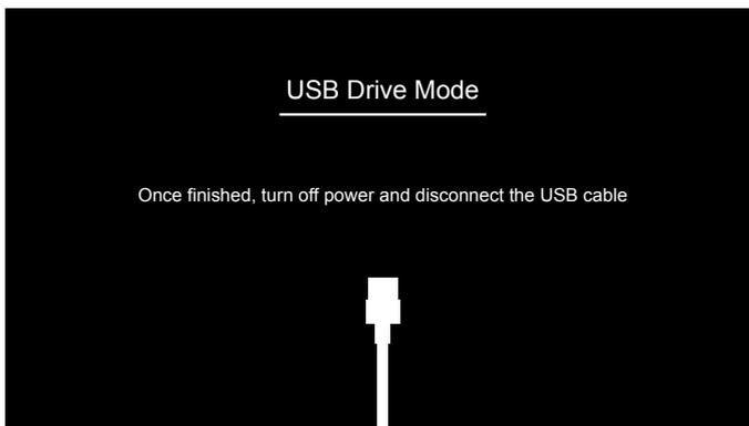
Once the 2 devices have been connected, power up your Maturmeat®. Your controller will now display the communication mode screen, and a new window will open on your computer. Copy/Cut the firmware file from its current location and paste into newly opened window. A small uploading window will appear and will take several seconds (depending on computer) to begin. Once completed, power down your Maturmeat and disconnect the micro USB cable from the controller.
